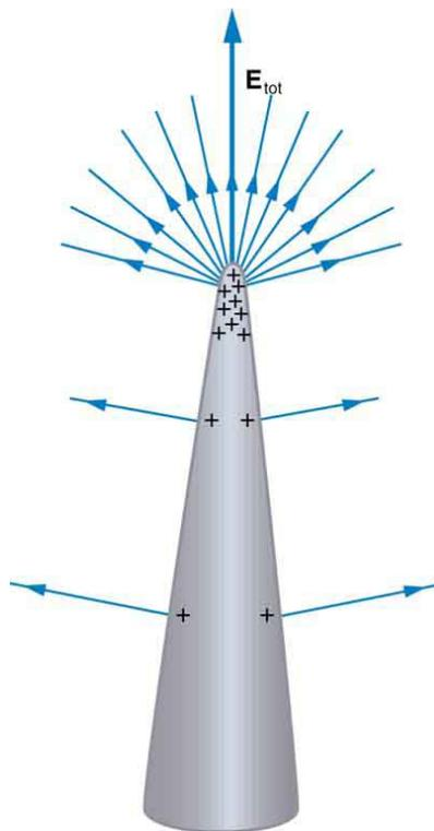
**Figure 18.36** A very pointed conductor has a large charge concentration at the point. The electric field is very strong at the point and can exert a force large enough to transfer charge on or off the conductor. Lightning rods are used to prevent the buildup of large excess charges on structures and, thus, are pointed.
