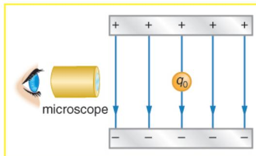
**Figure 18.58** In the Millikan oil drop experiment, small drops can be suspended in an electric field by the force exerted on a single excess electron. Classically, this experiment was used to determine the electron charge  $e$  by measuring the electric field and mass of the drop.
